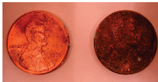
Figure 10. Coated (left) and uncoated (right) pennies after 24 h exposure to 5% NaOCl solution.
